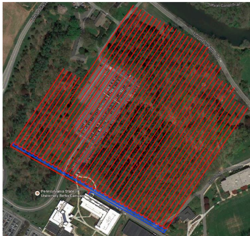
Figure 23: Proposed configuration of the Gaige Building's horizontal loop geothermal system
