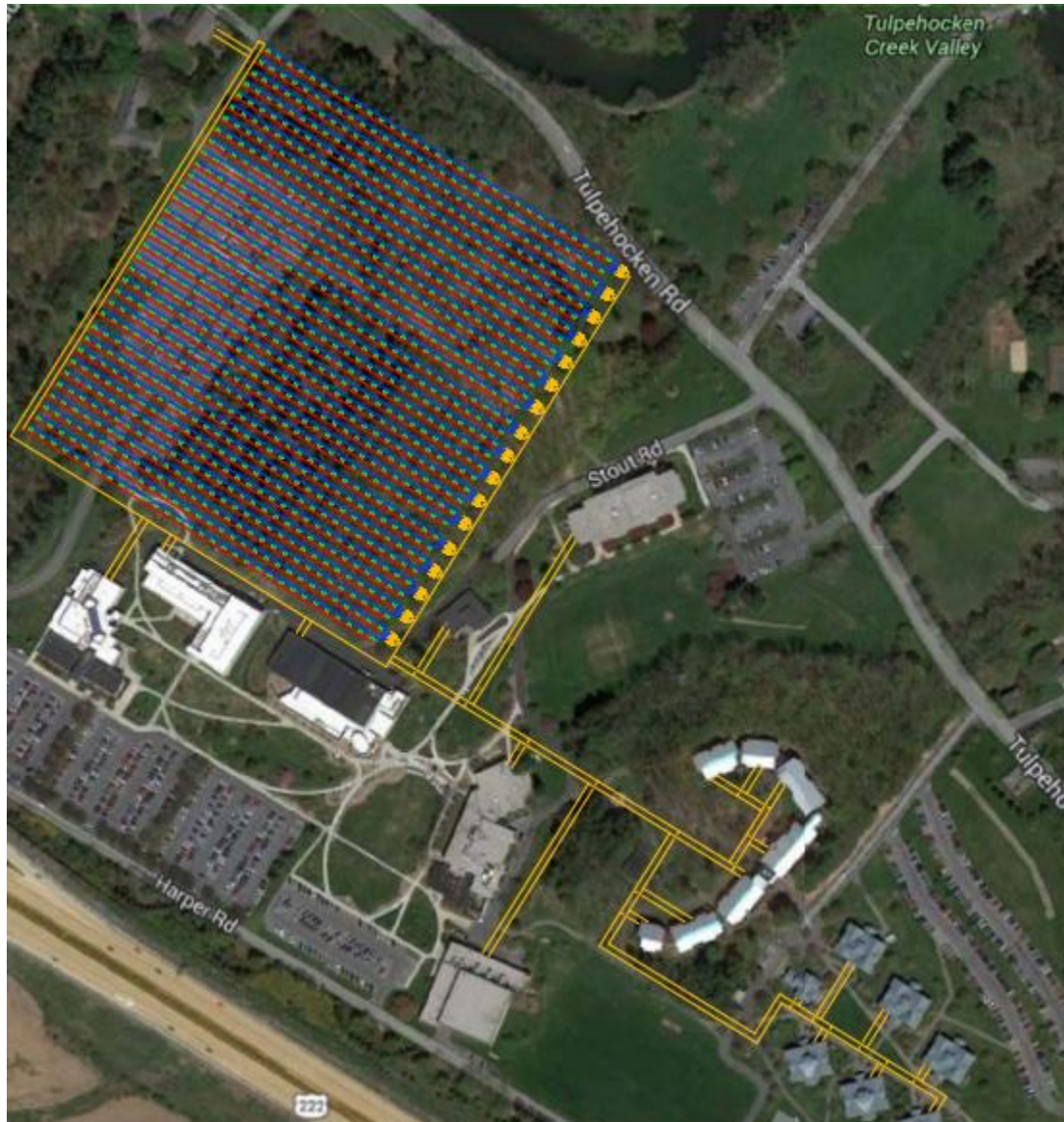
Figure 50: A layout of the overall geothermal system to serve the campus. Well field piping is shown in blue and red, and orange piping is part of the campus distribution piping. Pumps are shown as orange boxes
